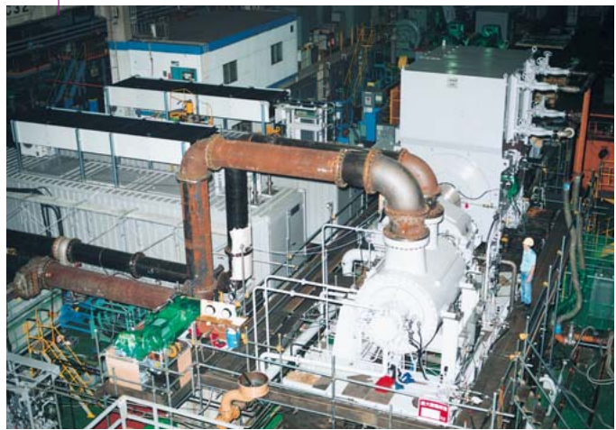
BCH804 Complete Unit Test with 35MW Motor
