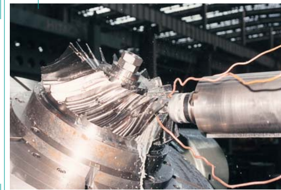
Five-Axis Machining of a Mixed Flow Impeller
